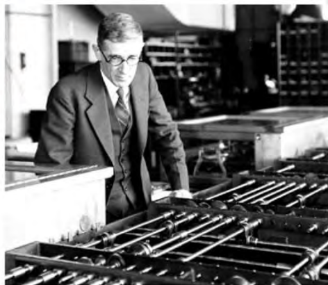
Vannevar Bush, during World War II, with his “differential analyzer” mechanical calculator at the Army’s Aberdeen Proving Grounds.
